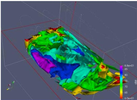
Figure 4. Set of 3D isosurfaces for sound in front of a Mackie HR824mk2 speaker playing a 1kHz tone, plotted using ParaView [7]. Here the 3D surfaces are sliced horizontally to reveal their structure. The variability and lack of symmetry may be due to drift errors or other location inaccuracies from the Tango system.
