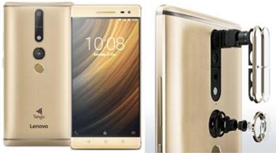
Figure 1. The Lenovo Phab 2 Pro, the first Google Tango device for the general public. The cameras and inertial sensors are used by the Tango software to provide a representation of the room and the phone's position within it. (Source: Lenovo.com)
