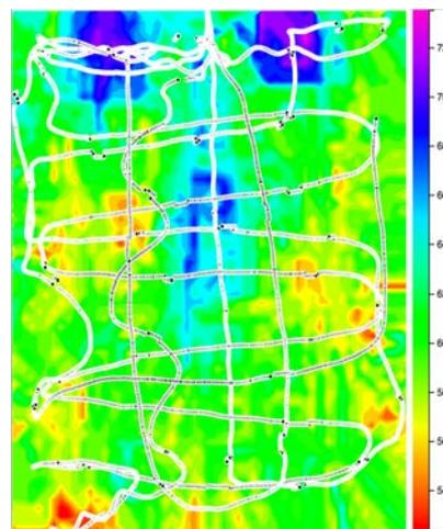
Figure 2. 2D contour plot of sound intensity level in Columbia Studio A, with pink noise played from a PA at the top of the figure.
