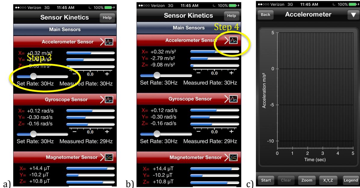
Figure 1: a) Set the sample rate as high as it will go, then b) press graph-arrow for the Accelerometer. Doing so will bring up the screen shown in c).
